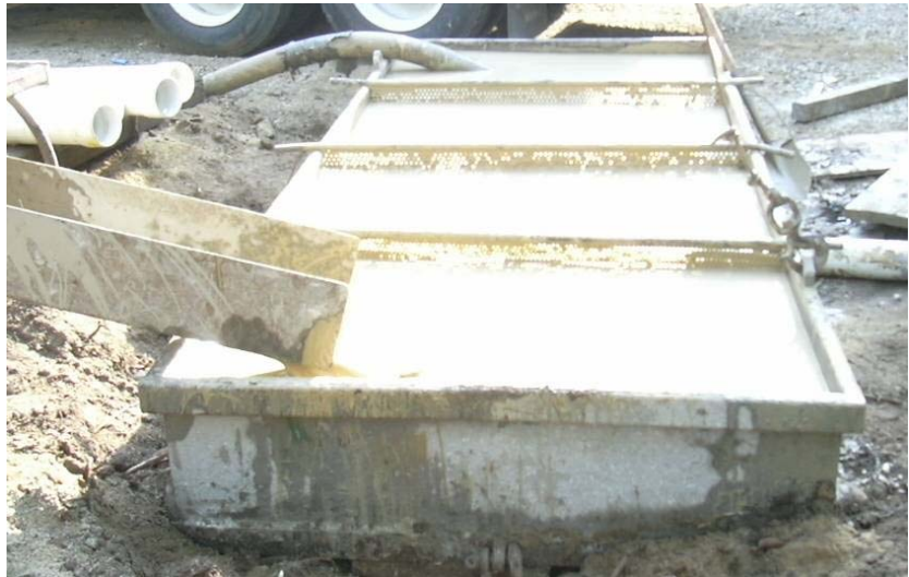
A typical above ground mud pit:
